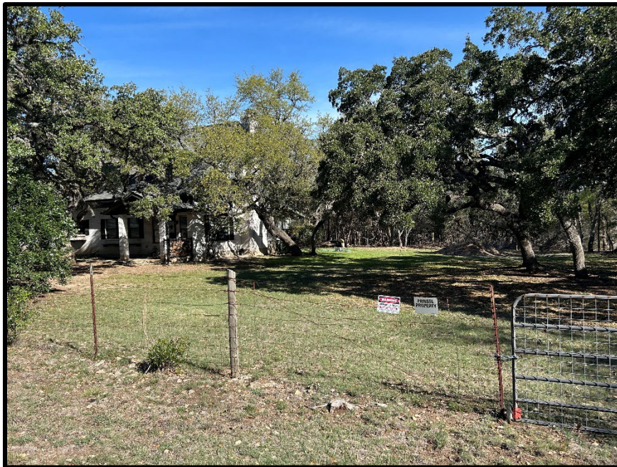
Figure 3: Although there are combustible materials within the Immediate Zone, the lack of ladder fuel, no wooden structures touching the home, and home construction all reduce risk while keeping desired landscape features.
