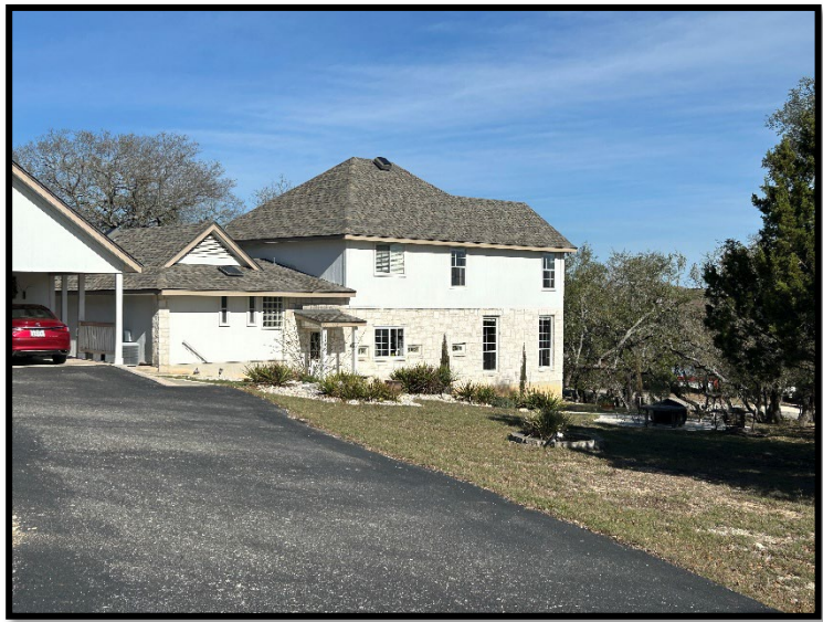
Figure 2: Xeriscaping reduces the chance of structure ignition by the reducing amount of fuel that is available to burn.
